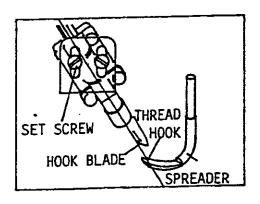
WHEN MOVABLE KNIFE MOVE FORWARD TO ITS LOWEST DEAD POINT, THE TIP OF THE MOVABLE KNIFE SHOULD LOCATE AT THE HALF DISTANCE BETWEEN SPREADER AND PRESSER FOOT. LOOSEN THE NUT OF CYLINDER, ADJUST THE PISTON TO ITS PROPER POSITION THEN TIGHTEN THE NUT.
